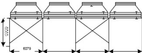
C3/C4 splitter condenser with thermal duty of 9875 KW
