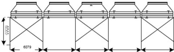
C3/C4 splitter condenser with thermal duty of 9875 KW
